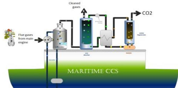
The underlying feasibility study is not in the public domain, but the press release reports that it would be possible to design a Maritime CCS system to capture of about 70,000 tonne per year CO<sub>2</sub> from a VLCC (very large crude carrier) class of vessel with over 50% capture efficiency. The CO<sub>2</sub> would be stored in dedicated tanks on board the vessel to be off-loaded at a suitable port.
